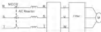
Figure 4.19 Wiring at motor side
